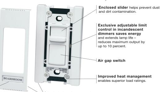
**Exclusive adjustable limit** control in incandescent dimmers saves energy and extends lamp life reduces maximum output by
