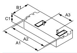
ELE BALLAST (2) 13W CFL (4-PIN) 120-277V
