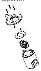
Round Single-Gang Floor Box Assembly – Includes singlegang box, one 15A, 125V tamperresistant duplex receptacle with two (2) USB charging ports, recessed 2" (51mm) below cover. Also includes round nickel cover with hinged access door and two (2) wire egress openings.
