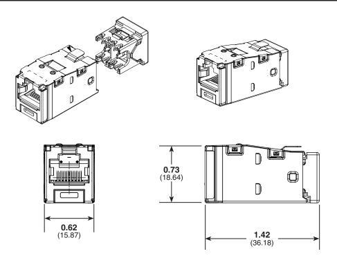
Dimensions are in inches (Dimensions in parenthesis are metric)
